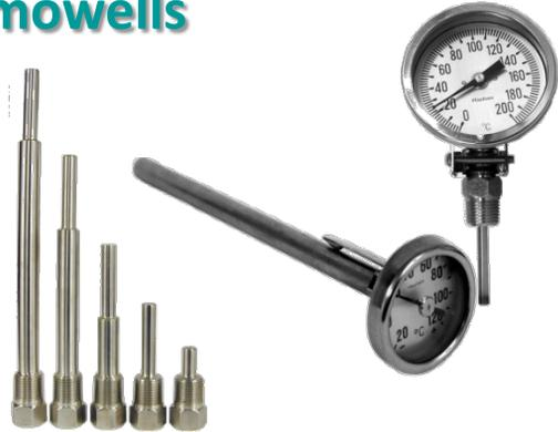
The CVS and Pfortner Thermowells can be used in a variety of different process applications where viscosity, pressure, corrosive, or abrasive materials are present. Thermowells allow removal of the temperature instrument for replacement, repair, or testing without contaminating the process media.
