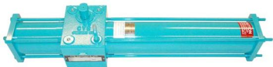
CVS 35D uses a scotch yoke mechanism for high break away and reset torques. Used for opening and closing quarter turn ball and butterfly valves.
