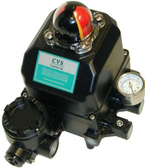
The CVS Electro-Pneumatic Positioner YTC-1000R is used for operation of pneumatic rotary valve actuators by means of electric control for systems pneumatic output signals of 3 - 15 psi or 6 - 30 psi.
