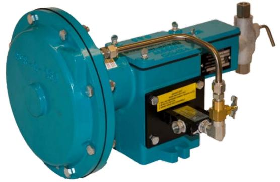
Supply pressures are 15 - 35 psi and the pump will operate at 0 to 30 strokes per minute with a 1 inch stroke. Available injection plungers are 3/16", 1/4", 3/8", and 1/2". The pump housing is constructed out of powder coated cast aluminum. Plunger packing material can be Buna-N, Viton, Teflon, or Flourosilicone. O-ring suction and discharge seals can be Buna -N, Viton, or Flourosilicone.
